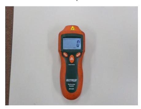
Hold the laser or light beam from the photo-Tachometer on the bottom edge of the exciter case while the vibratory hammer is vibrating
